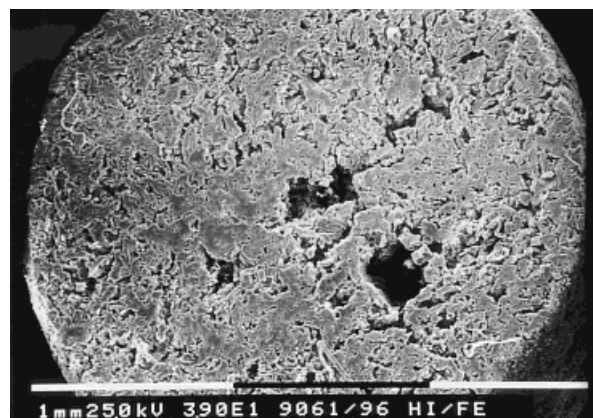
Figure 1 Scanning electron microscopy (SEM). The section of a polypropylene porous particle.
